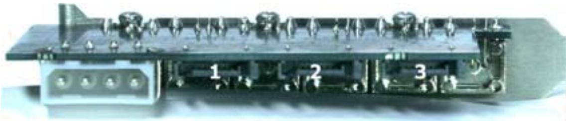
The three SATA ports on the CMI card are shown here. They should be connected to the ports of the same number on the CC-1 card, shown below.
