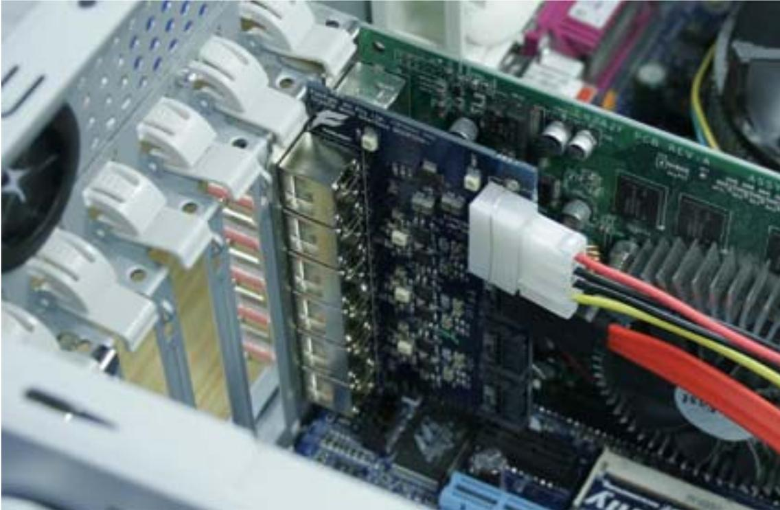
Step 3 Connect three SATA cables from the CMI board to the CC-1, keeping the numbering aligned.
