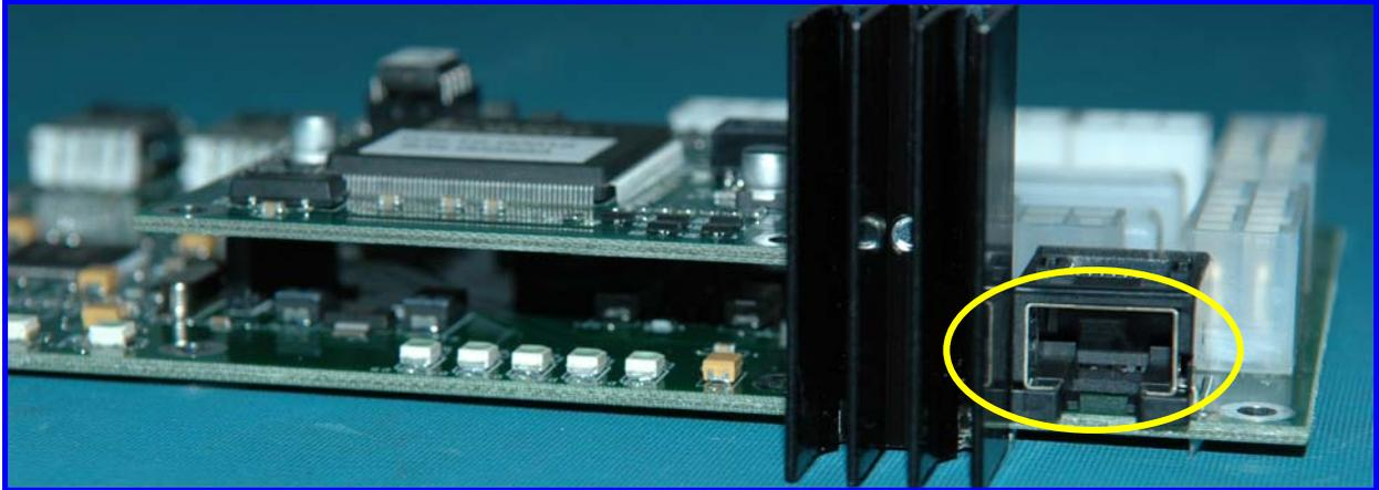
Rear view of the BMIX002A circuit board, showing the RJ-45 connector at the right.
